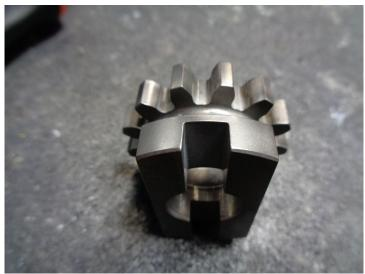
If you install the gear incorrectly you will not be able to time the MAG to the engine, because you will MAX OUT the Ear Slots on the mag BEFORE getting a POINT BREAK.
