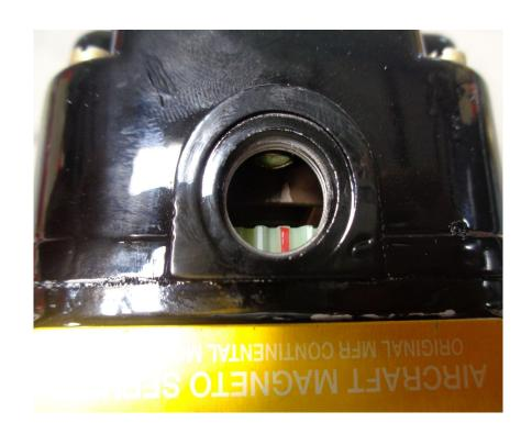
3) With the Mag on the bench, timing window facing the ceiling RED PAINTED TOOTH in the window, Shaft pointing at you, the Impulse Coupling body has Two raised areas that the Drive Gear engages. One is located at the 4 O'clock position and the other at the 10 O'clock position.
