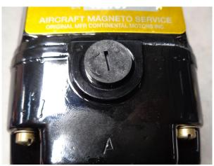
2) The mag direction of rotation is always viewed from the shaft of the magneto. Turn the mag backwards, (clockwise, so that we are not winding up the impulse coupling spring) until you see the RED PAINTED distributor gear tooth enter the timing window. Continue to turn the Shaft until you feel magnetic NEUTRAL (the mag will want to hold this position), and the RED PAINTED tooth will be offset in the window.
